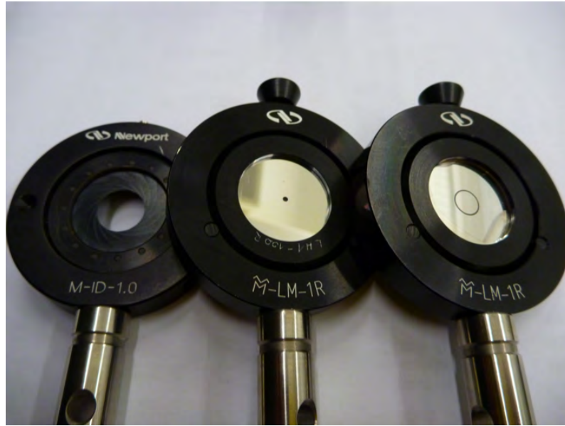
Fig. 39: Three different apertures to modulate the incident angle. Left: FF, middle: PAR, right: MR.
